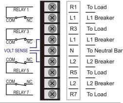
13) Make 12VDC connections through the rectangular knock-out located in the back of the box per the diagram on the right and pin-out below.
